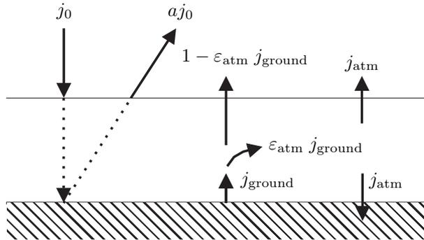
Figure 13.1: The illustration to the solution of the 6<sup>th</sup> problem.
