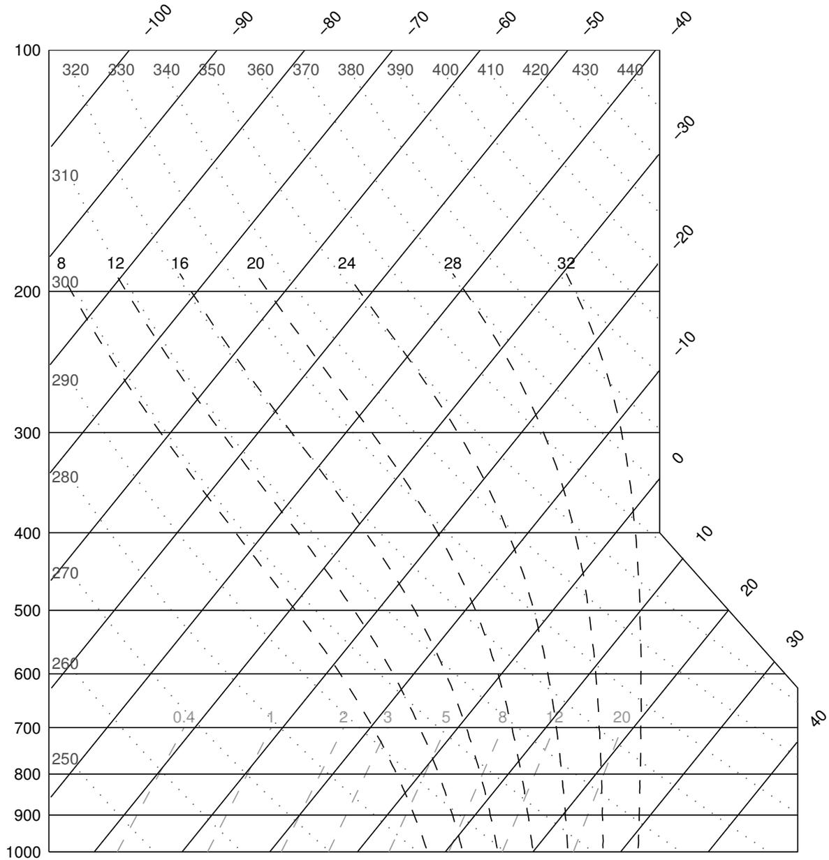
Figure 15.1: Empty Skew-T Log-P emagram.
